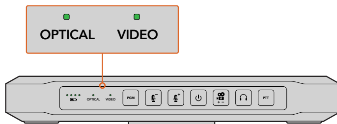
When a valid video signal is detected via SDI or HDMI, you'll see ATEM Camera Converter's 'video' status indicator illuminated. The 'optical' indicator will illuminate when a valid SDI signal is detected via the optical fiber input.
