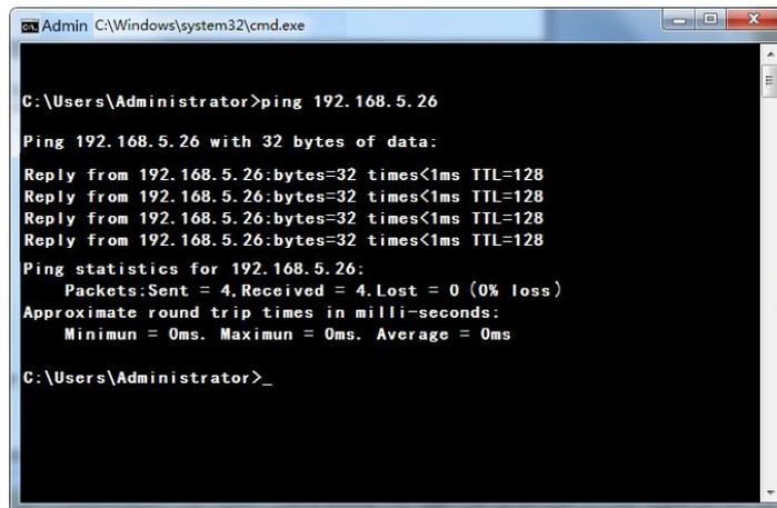
5) User can also to verify network connection as steps above mentioned after the finish of camera self-check. If IP is default, open DOS command window and input 192.168.5.163,then press Enter key. It will show message as below: which means network connection is normal.
