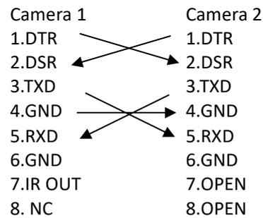
**Note:** PTZ Camera has RS232 input and output interface, so you can cascade as the above way.
