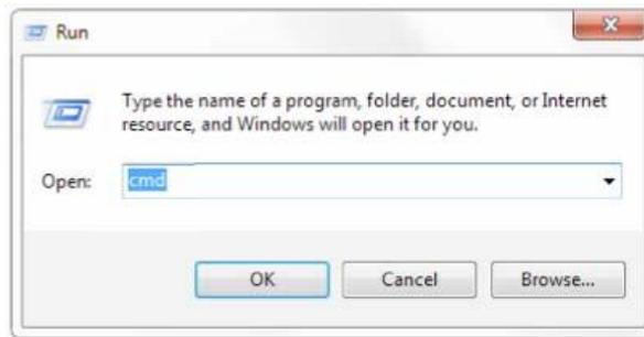
4) Click "OK" and open the DOS command window, input ping 192.168.5.26 and press Enter key, it will show message as below:which means network segment adding is succeed.
