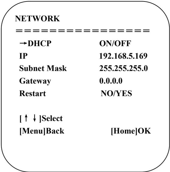
**DHCP:** options: ON/OFF; Turn off DHCP to set the IP address, subnet mask and gateway (NOTE: must be in the same network segment as the IP address).
