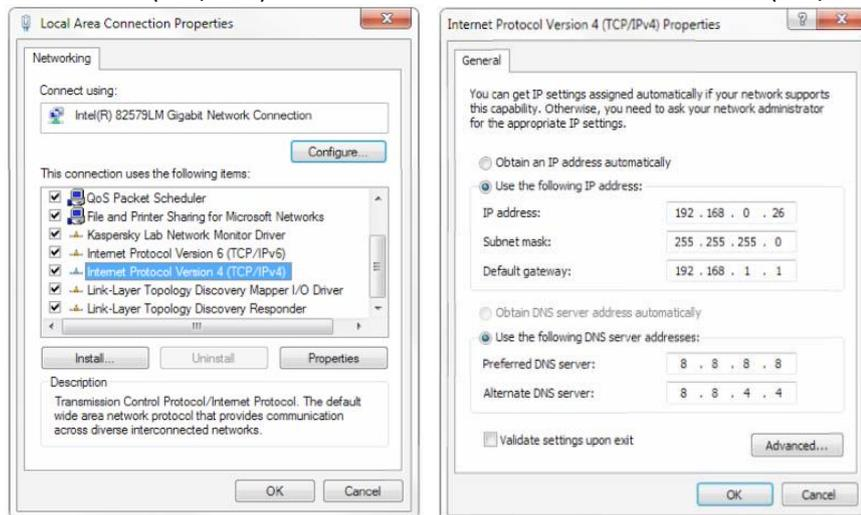
2) select “Advanced” to enter into the Advanced TCP/IP Setting and add IP and subnet mask in the IP browser as picture shown below. Click the “Confirm” to finish the adding of IP segment. User can add the corresponding network segment according to the revised IP address of the camera.
