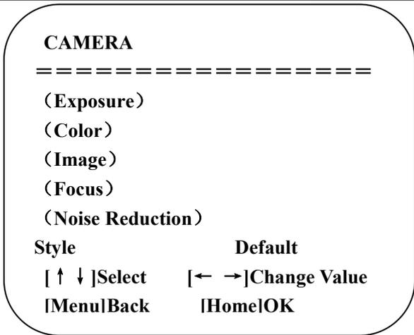
**Exposure:** Enter into Exposure setting      **Image:** Enter into image setting      **Color:** Enter into color setting
