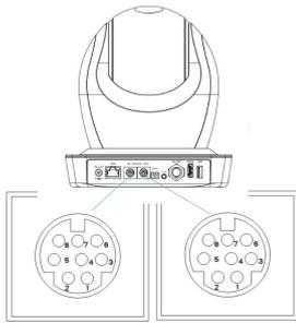
Computer or keyboard and camera connection method
